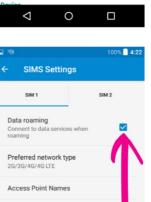
Tap the empty check box to the right of "Data Roaming". Read the warning and click "**OK**". This will put a blue check in the "Data Roaming" box.
