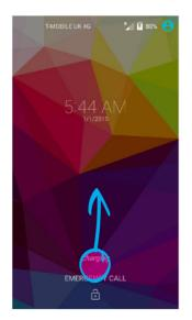
Press the power button located on the top of the right edge of the phone (under the volume buttons). Unlock your phone by dragging the padlock symbol upwards.
